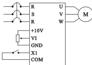
参数设定: Pr033=1 Pr034=1 Pr066=50 Pr068=50
